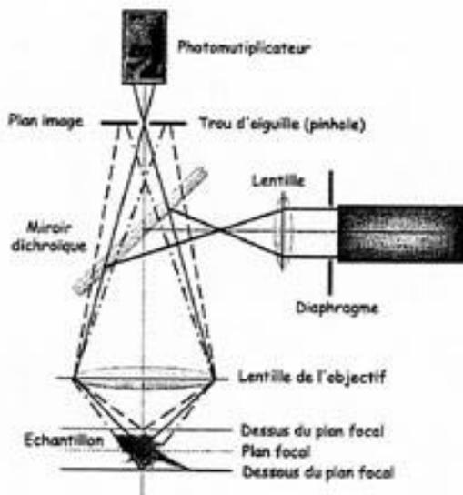
Figure 7-2. The single-photon laser-scanning confocal microscope.
