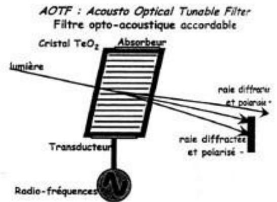
Figure 7-3. A gem for microscopy, the AOTF.
